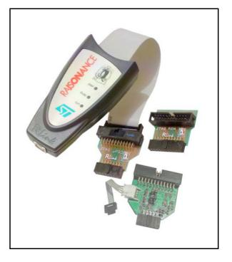
The RLink does not include trace support for ARM® core-based devices with Embedded Trace Macrocell<sup>™</sup> such as STR9. Tools with trace capability are available in the STR9 Professional Developer Kit from Raisonance (STR9-DK/RAIS) with Signum JTAGjet, and in the STR91x Advanced Developer's Kit from IAR (STR91X-DK/IAR) with J-Trace.
